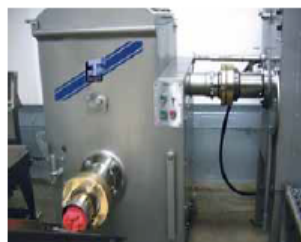
Standard 4000 Model 15 kW - 2 Speed Mince - 56 Head Gemini Connection - available to various machines
