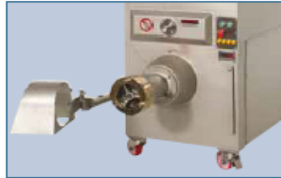
Illustrating 4200 Frozen 4 Speed Inverter Feedscrew Controller with Digital Readout
