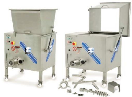
900 MIXER MINCER WITH SAFETY INTERLOCKED HOPPER EXTENSION FOR AUTO LOADING (OPTIONAL)
