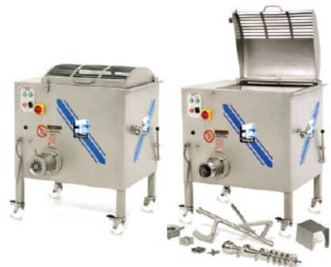
900 MIXER MINCER WITH SAFETY INTERLOCKED DOME LID (STANDARD)
